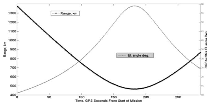
Figure 4. OGS to Nfire Range and Elevation engagement characteristics for the 14<sup>th</sup> of July 2010, starting at 23:27:00 UT.
