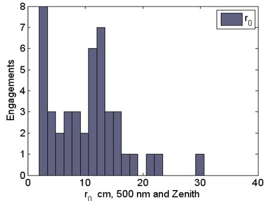
Figure 2. Number of link engagements with a mean Fried Coherence length ( $r_0$ ) for the engagement plotted as a function of the Fried Coherence lengths. The means are averaged over the engagement length from the University of Hawaii, Haleakala monitor which measures and reports at zenith, 500 nm and 1 minute intervals.
