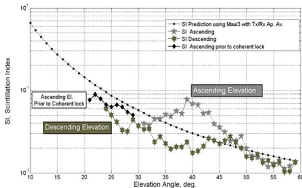
Figure 6. Measured FAS SI and predicted SI plotted against elevation angle. The predicted SI uses the Maui 3 model and takes into account receiver and transmitter aperture averaging. Three regions highlighted in this plot; 1<sup>st</sup> ascending elevation prior to coherent lock, 2<sup>nd</sup> ascending elevation during bidirectional communication and 3<sup>rd</sup> descending elevation also during bidirectional communication.
