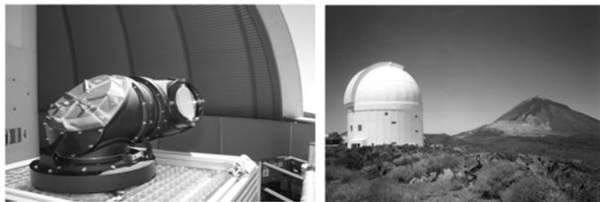
Figure 3. The ground LCT mounted in the ESA-OGS dome in Izana, Observatori del Teide. The left image shows the LCT resident in the dome of the ESA-OGS. The dome slit is in the upper right of the left image and was programmed to move with the azimuth movement of the LCT.
