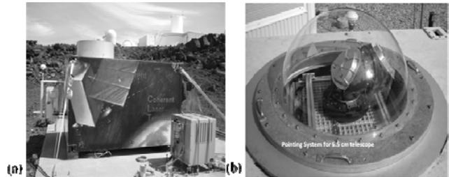
Figure 1. (a) Container on Haleakala with metal protective cover over the ground LCT. (b) Engagement ready LCT on AMOS except for removal of plexi-glass cover.
