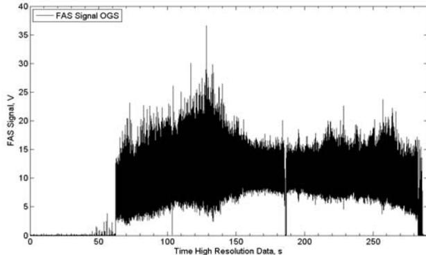
Figure.5. High resolution data for the OGS received FAS signal plotted against mission time. The dropout at 186 seconds is due to a physical obscuration inside the dome. Note that both NFIRE and the ground LCT remained locked through this fade.
