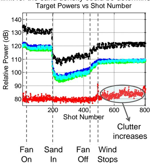
Figure 4. Time resolved return powers from various targets along with the noise floor (see text).
