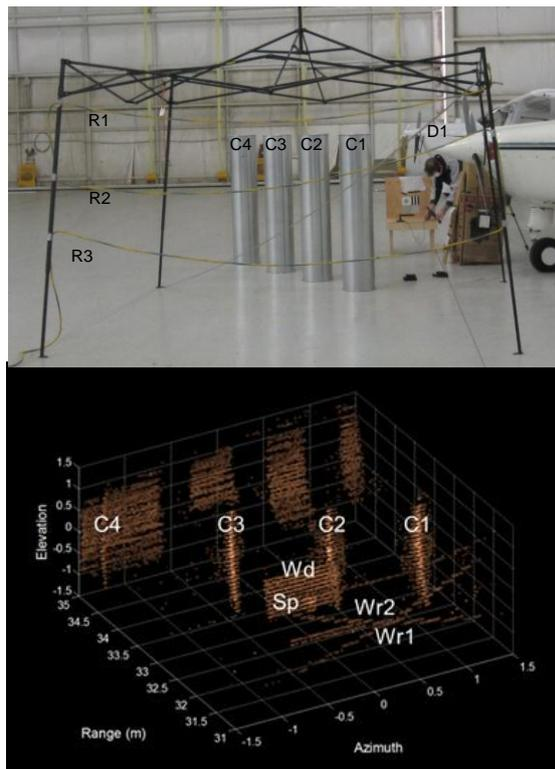
Figure 7. (Top) Typical test scene. (Bottom) 3D point cloud obtained from ~35 m using Bridger's system.
