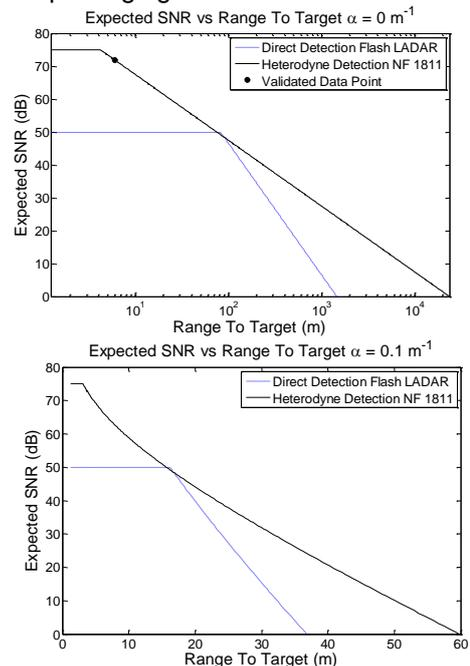
Figure 1. Expected SNR versus the range to the target for the DD and HD cases described in the text with (Top) no atmospheric attenuation and (Bottom) the atmospheric attenuation experienced during the Yuma Proving Ground tests. In both cases, the HD system is capable of seeing substantially further than the DD system.
