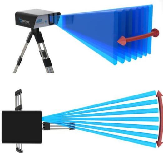
Figure 2. (Top) A view of the 3D imager and the output beam. Information imaged in elevation via a one dimensional focal plane array and in azimuth via a proprietary non-mechanical scanning method and in downrange via FMCW ladar resulting in a true angle-angle-range image. (Bottom) A view from the top showing the azimuth scan angle.
