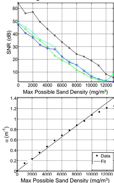
Figure 6. (Top) The minimum SNR seen versus maximum possible sand density supported by the brownout chamber. See text for target coloring which is the same as Figure 4. (Bottom) The measured extinction coefficient.
