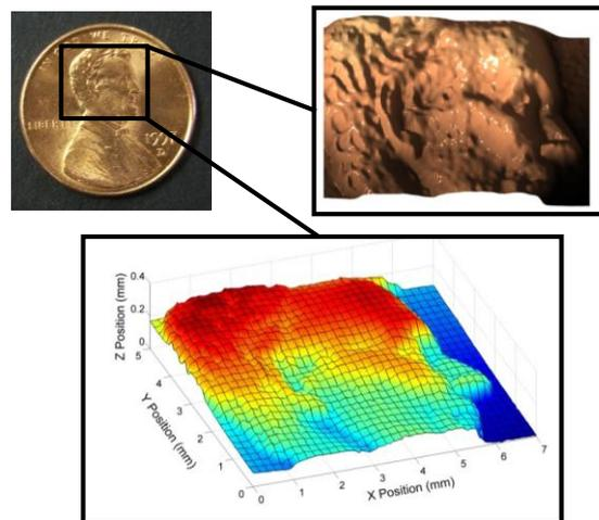
Figure 3. (Top Left) The approximate location of the scanned section for a U.S. Penny. (Top Right and Bottom) Renderings of the three dimensional imagery acquired with the swept source.
