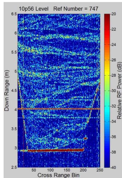
Figure 5. Wisps of the sand imaged when the wind velocity is dropped nearly to zero in the sand chamber. The front of the chamber is visible near 3 m and the side walls are diagonal lines stretching upwards. The signal at 4 m is a noise spur.
