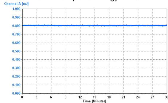
Figure 3. Pulse energy as a function of time. The fluctuations were 0.34% of the mean pulse energy.
