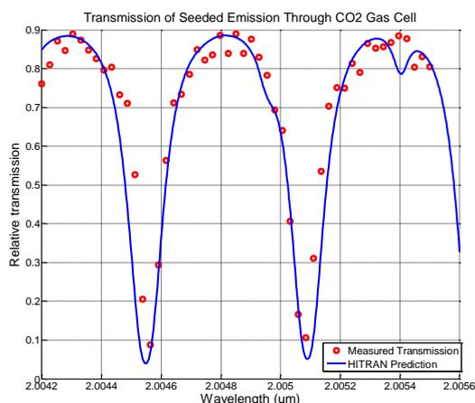
**Figure 5. Relative transmitted pulse energy as a function of wavelength.**
