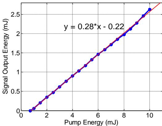
Figure 1. Output signal pulse energy as a function of input pump pulse energy for a 35-mm PPCLN crystal.
