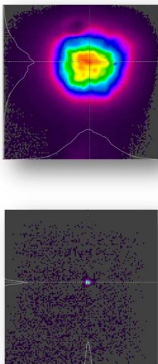
Figure 2. Top: Unfocused output from our parametric source at the idler wavelength. Bottom: The same beam after focusing with a 50 mm lens to obtain a beam diameter
