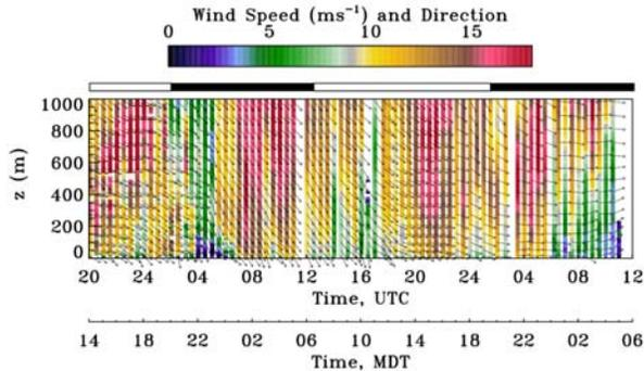
Figure 3. Time-height cross section of mean wind speed and wind direction. Horizontal axis is hour UTC and MDT. Wind speed is color coded from 0 to 18  $\text{m s}^{-1}$ , and wind direction is shown by black arrows. The bar below the color scale shows local daytime (white) and nighttime (black) hours.
