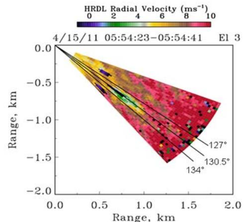
Figure 5 Enlarged and annotated sector scan of Fig. 4 (left, top). Solid lines indicate range of azimuth angles (127°-134°), and azimuth of a turbine location (130.5°).
