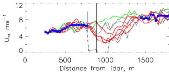
Figure 6 Propagation of the horizontal velocity, measured along several azimuth angles as indicated on Fig. 5. The horizontal axis is the distance from the lidar. The black solid line indicates the location of the wind turbine at 130.5° and 891 m from the HRDL.
