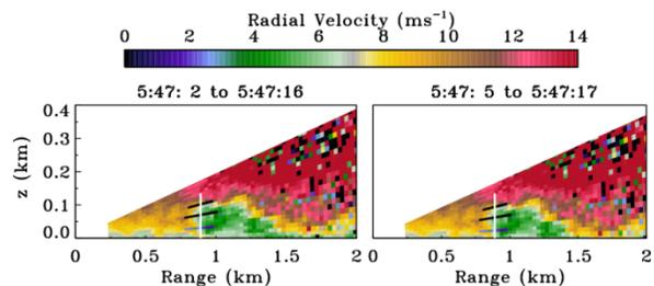
Figure 2. Vertical-slice scans, performed  $0.5$  degree off the HRDL/turbine direction, illustrate velocity deficit downstream of the wind turbine, as shown on the plot by white vertical line. The horizontal axis is the distance from the lidar.
