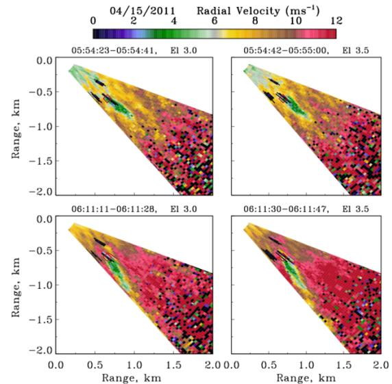
Figure 4 Sector scans performed at 3° (left) and 3.5° (right) elevation and within range of azimuth angles of 112°-145°. Horizontal and vertical axes are distance from lidar in km. Wind speed is color coded from 0 to 12  $\text{m s}^{-1}$ .
