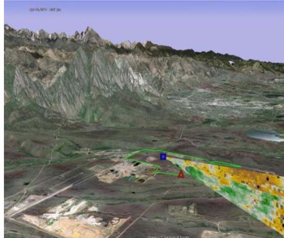
Figure 1. A vertical-slice scan, performed at  $1^\circ$  to the north of the azimuth to the turbine at shallow elevation angles, superimposed on a Google Earth image of the study area. The green line indicates the boundary of the experimental site. Locations of the wind turbine and the HRDL are shown by the red triangle and the blue square respectively.
