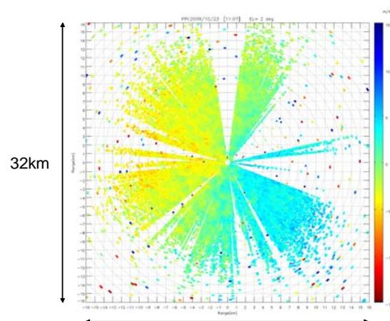
Figure 2. PPI measurements of horizontal winds (EL=2 degree)
