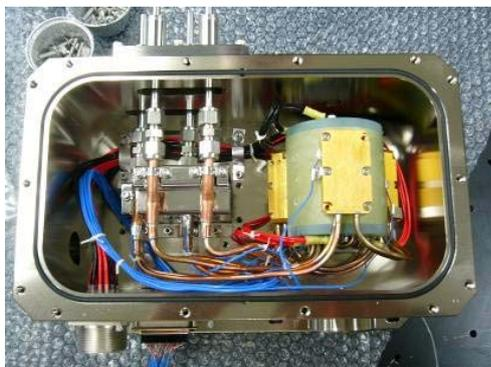
Figure 4 new laser head in a vacuum container
