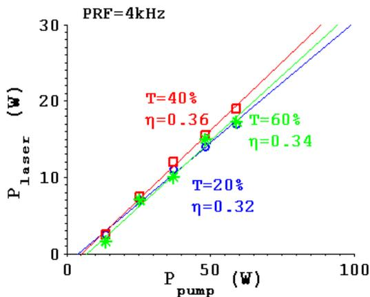
Figure 2. Laser output power versus the pump power at 2051 nm, PRF=4 kHz, using different output couplers
