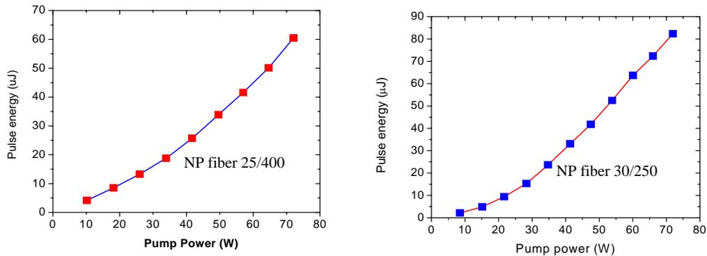
**Fig. 3** Pulse energy results at 1572 nm for two NP fibers in the 2<sup>nd</sup> power amplifier stage at different pump power levels
