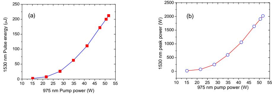
**Fig. 2** (a) Output pulse energy of the 2<sup>nd</sup> power fiber amplifier at different pump power; (b) Output peak power of the 2<sup>nd</sup> power fiber amplifier at different pump power.
