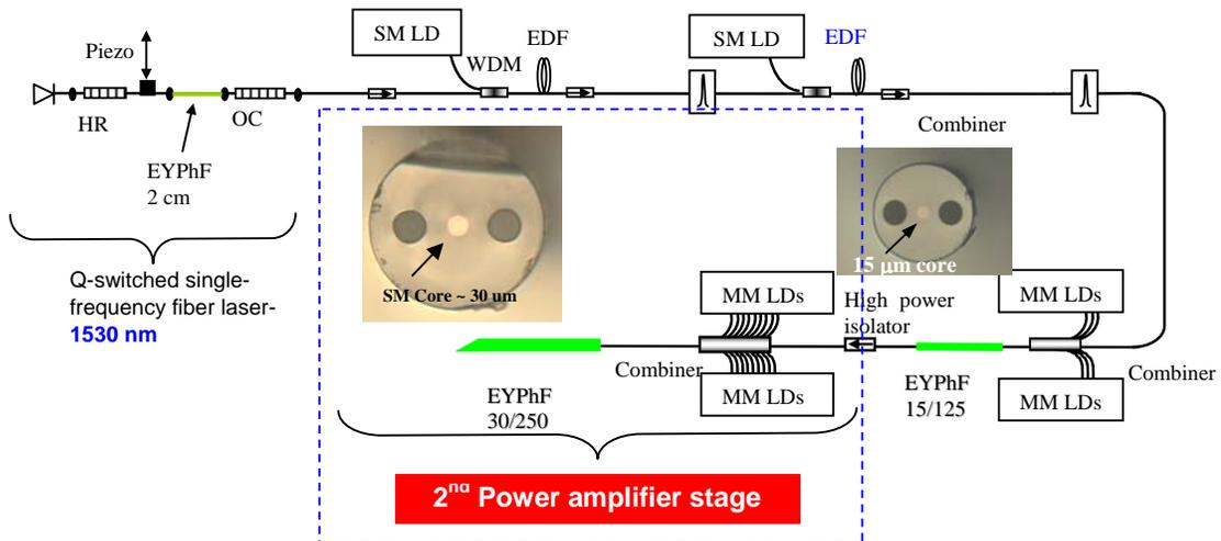
**Fig. 1** Schematic of the monolithic Q-switched pulsed fiber laser based on the new large core highly Er/Yb co-doped phosphate fiber 30/250.
